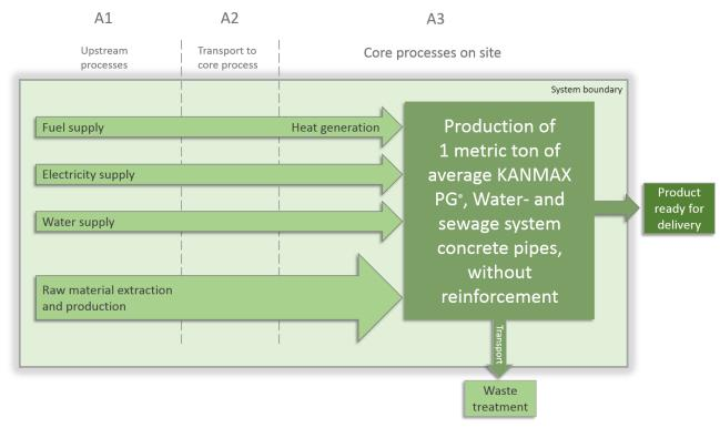
Figure 2. Flow diagram of the assessed life cycle stages for KANMAX PG®, beginning with raw material extraction and production, followed by transport from supplier to site and finally manufacturing at the core sites.
